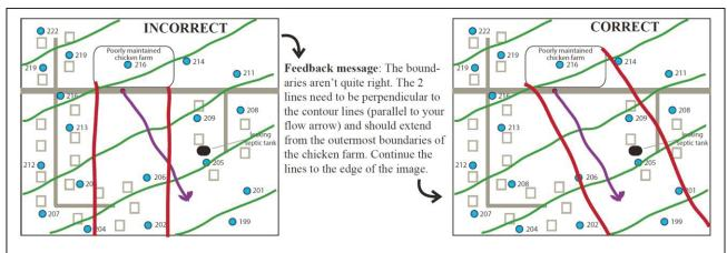
Figure 1: Example of student work on a groundwater contamination worksheet. Contour lines (green) and flow paths (purple and red) are difficult concepts for students, so drawing them and the flow paths are useful. On the left is a common student mistake, in the middle is the feedback from the worksheet, and on the right is the student's corrected sketch.
