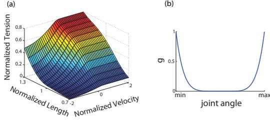
Fig. 3. (a), The total force produced by a muscle fiber at a given level of activation depends on both its instantaneous length and velocity, which are independent kinematic variables. (b), polynomial function to punish moving towards joint limits.
