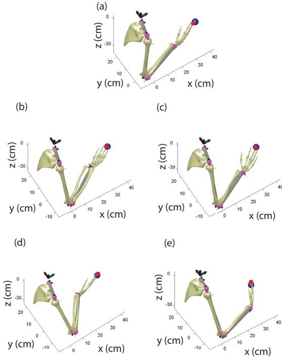
Fig. 7. Arm configuration with the same end-effector position but different palm orientations. (a), wrist is not bended. (b), positive pronation-supination of the wrist. (c), negative pronation-supination of the wrist. (d), positive flexion-extension of the wrist. (e), negative flexion-extension of the wrist.
