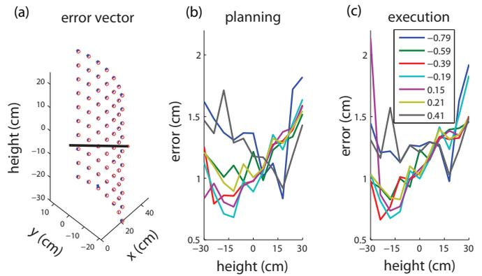
Fig. 6. Endpoint errors in reaching movements. (a), Target locations and the corresponding error vectors. Each target location is determined by two parameters: height and angle on the x-y coordinate. (b), Endpoint positional errors planned by the high-level controller. (c), Endpoint positional error executed by the low-level controller. Lines with different colors represent errors from movements towards targets with different angles.
