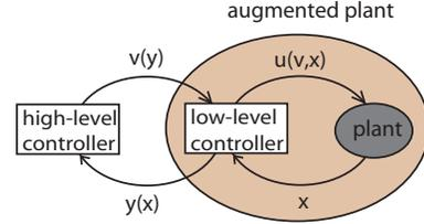
Fig. 1. Schematic illustration of a hierarchical control framework [2].
