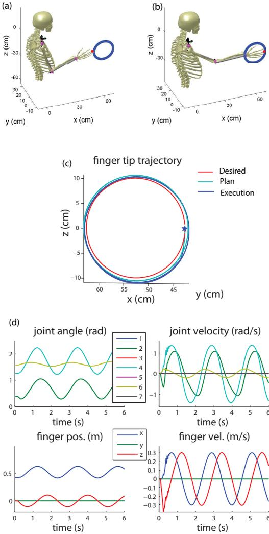
Fig. 9. Arm movements during drawing. (a) (b), arm configuration at the beginning of and during drawing. (c), end-effector trajectory during both planning and execution. (d), end-effector position/velocity in Cartesian hand coordinates, and joint angle/velocity in joint coordinates.
