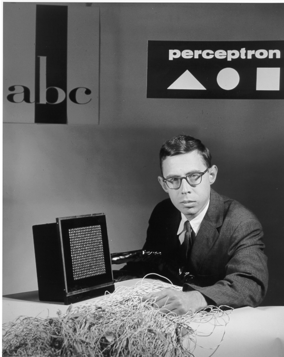
Figure 5. Frank Rosenblatt, originator of the perceptron, c. 1959. Here, he was photographed, in connection with a television appearance, with the ‘eye’ (a 20 x 20 array of photoconductors) of the “Perceptron Mark I” pattern recognition neurocomputer. Note that the bundle of 400 wires in front of Rosenblatt, which make up the ‘optic nerve’ of the perceptron’s visual system, are “randomly scrambled”. The fact that the perceptron could adaptively learn to correct for such imprecise connections was one of its many appealing attributes. The widespread publicity of Rosenblatt’s work, and that of his followers, stimulated (both in the press and among some researchers in the field) what might now be called an “irrational exuberance” regarding the prospects for rapid progress in the field of neural networks. This unwarranted exuberance, along with the widespread public attention, viscerally irritated and enraged a group of academics who (incorrectly, as it turned out) viewed themselves, and their ideas, as far more worthy of such optimism and attention. Before long, this group launched a vicious and brutal, but well-calculated and highly successful, attack against Rosenblatt in particular, and the field of neural networks in general. Rosenblatt’s career declined and research on neural networks almost stopped for twenty years. Photo courtesy of Veridian Engineering.
