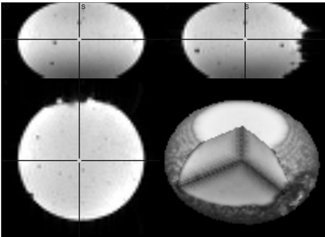
**Figure 2** Results of the BIRN test for the fully shielded robot with movement. The three images with crosses show sections of the spherical head model, and the bottom right shows a three dimensional view. The small dots are bubbles in the static head model and are always present. The lack of large stripes or zippers indicates that the noise from the robot is uncorrelated.
