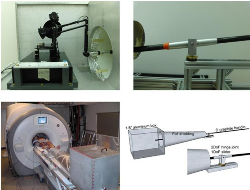
**Figure 1** The apparatus used to mount the haptic robot for use in the fMRI environment. Top shows the haptic robot mounted in the case prior to enclosure (top, left) and the gimbal/slider joint at the midpoint of the handle (top, right). Bottom, left shows a subject in the scanner manipulating the handle. Bottom, right is a cartoon of the shielding and end effector.
